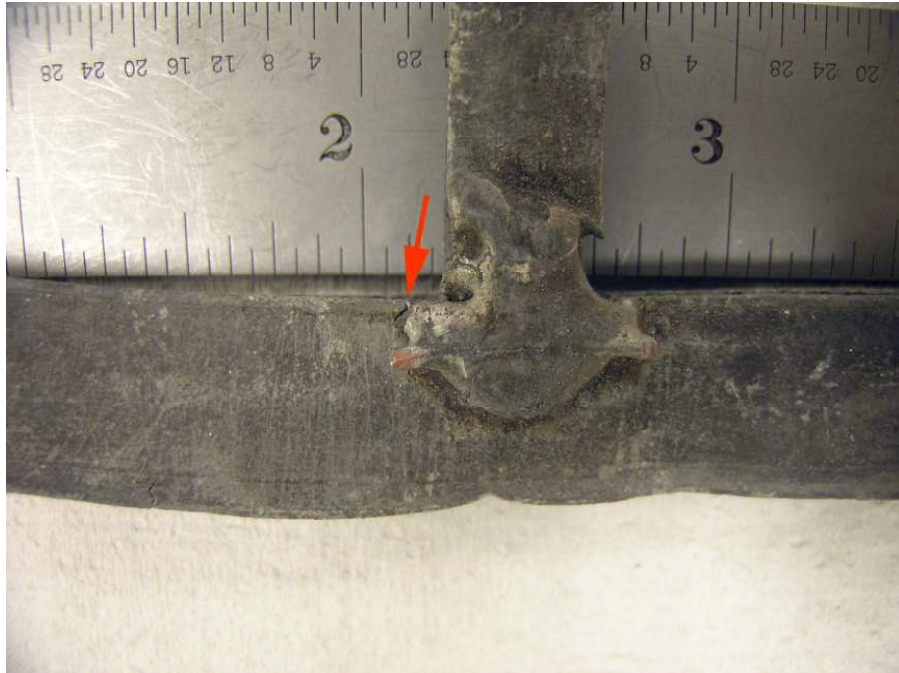
Figure 3: Close-up of crack in top joint of Figure 2, arrow. Note also joint profile and appearance.
