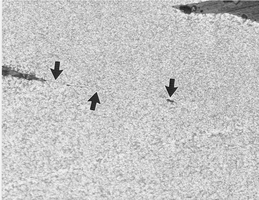
Figure 18: Higher magnification view of lack of fusion in Figure 17, arrows. As-polished. Mag. 100X
