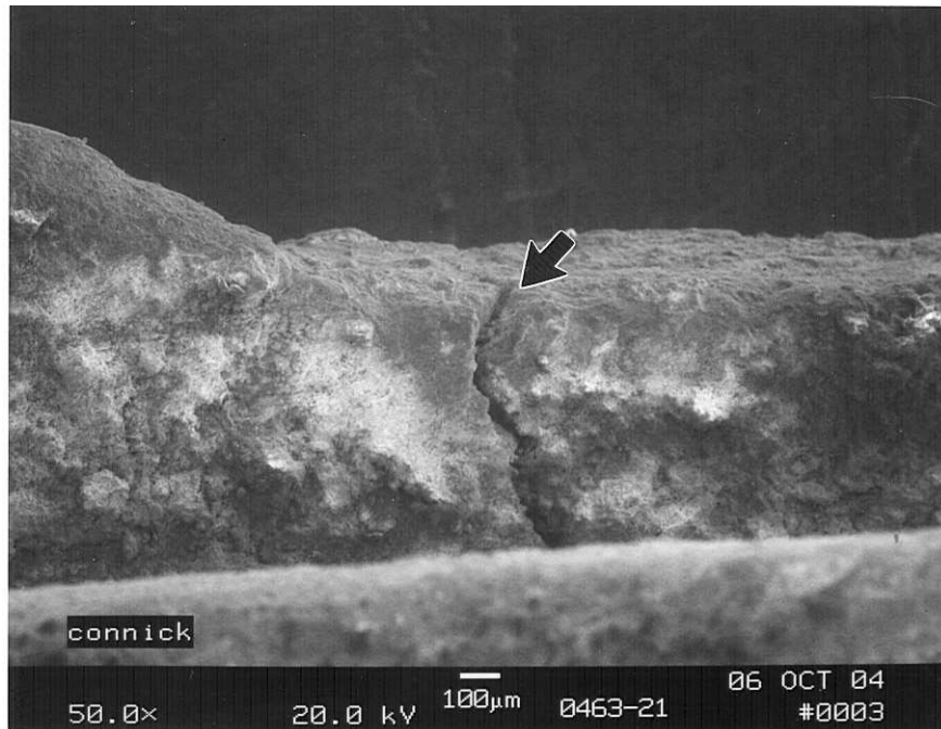
Figure 10: Crack in came near solder, Sample A, arrow. Mag. 50X
