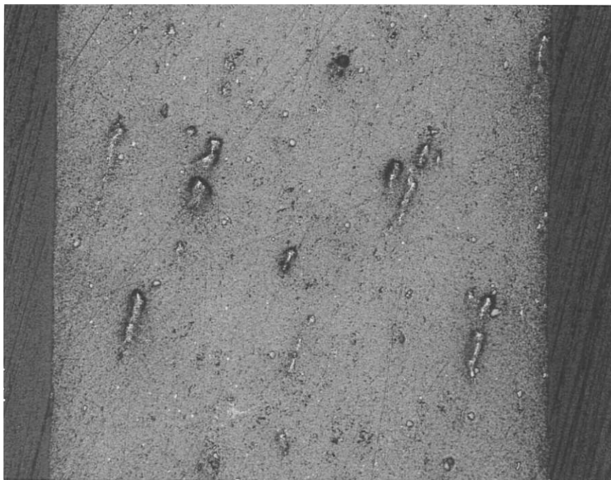
Figure 19: New came in cross-section. As-polished. Mag. 120X
