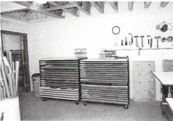
DISASSEMBLED WINDOWS —are neatly stored in 'baker's rolling racks'.
