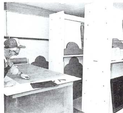
RUBBING —of the leading patterns of windows undergoing restoration, prior to disassembly, is made in the 'dirty room.'
