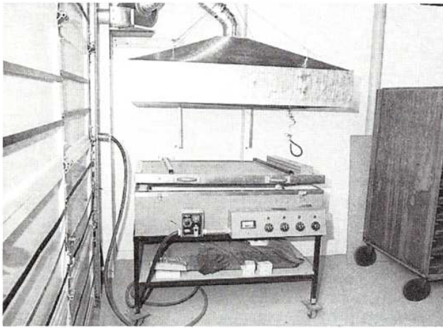
VENTED KILN —heavy metal fumes generated during firing are removed from the work area by a hood on a pulley system.
