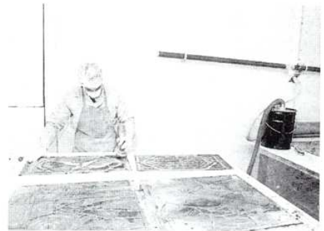
CONTROLLING DUST —during the cementing process is a vital part of studio lead abatement.
